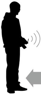
1. Turn on the transmitter first and then the vehicle.
